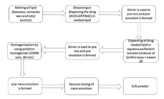
Fig 3: Schematic representation of SLN preparation by lipid extrusion (Castelli et al., 2005)
